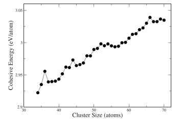
FIG. 8. Cohesive energies of neutral aluminum clusters obtained from the DFT calculations. The corresponding experimental results cannot be obtained with the present experimental method.
