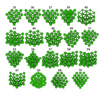
FIG. 7. A selection of cluster anion structures. The number of atoms in the cluster is shown on top of each structure. The structural families identified here are the same as for the cluster cations (Ref. 18): ddf around 36 and 53 atoms, disordered isomers around 46 and 66 atoms, and fcc-like fragments (with or without sf) for the rest of the sizes. The disordered isomers for n=45 and 46 (which are not shown in the figure) are nearly degenerate with the ordered global minima.
