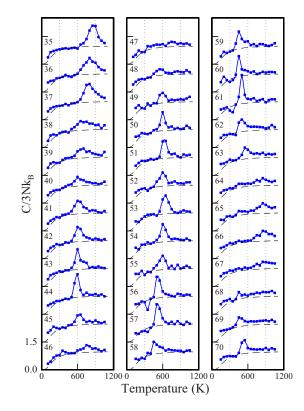
FIG. 1. Heat capacities recorded as a function of temperature for aluminum cluster anions with 35–70 atoms. The heat capacities are plotted relative to the classical value  $3Nk_B$ , where 3N=3n-6+3/2 and  $k_B$  is the Boltzmann constant. The filled (blue) squares are the experimental measurements. The solid (blue) lines running through the points are spline fits. The thin black dashed line is the heat capacity derived from a modified Debye model (Ref. 29).
