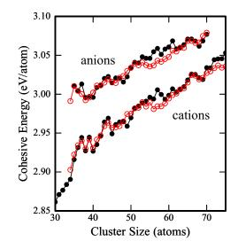
FIG. 6. Cohesive energies for aluminum cluster anions compared to corresponding results for the cations (Ref. 18). The filled black points show results derived from experimental measurements. The unfilled (red) points show results obtained from calculations using DFT.
