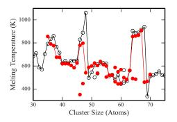
FIG. 4. Plot of the melting temperatures determined for aluminum clusters. The filled (red) points show results for the anions and the unfilled points show results for the cations (the data for the cations are taken from Ref. 13). Where there are two well-resolved peaks in the heat capacities (i.e., for  $Al_{46}^-$  and  $Al_{65}^-$ ) we show values for both transitions.
