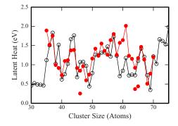
FIG. 5. Plot of the latent heats determined from the heat capacities for aluminum clusters. The filled (red) points show results for the anions and the unfilled points show results for the cations (the data for the cations are taken from Ref. 13). Where there are two well-resolved peaks in the heat capacities (i.e., for  $AI_{46}^-$  and  $AI_{65}^-$ ) we show values for both transitions.
